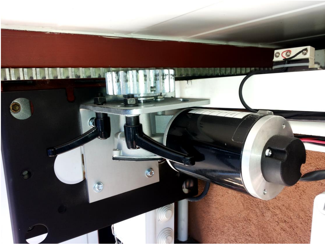
Motor and support with quick release system
